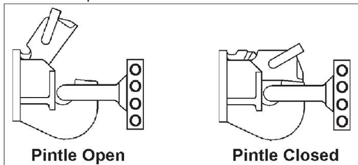
4. See the coupler instructions for details of placing the pintle in the “open” position.
