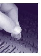
When they appear "even" with the outside of the tread, it is time to replace your tires. Another method for checking tread depth is to place a penny in the tread with Lincoln's head upside down and facing you. If you can see the top of Lincoln's head, you are ready for new tires.
